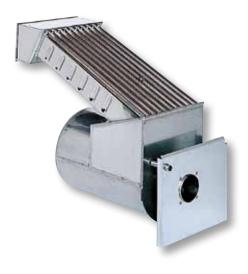
Patented highest efficiency heat exchanger, with air flow completely in counter current to the exhaust flow, made exclusively in 18% chromium stainless steel, which guarantees total protection against corrosion both from humidity and combustion by-products.
