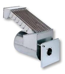
Patented highest efficiency heat exchanger, with air flow completely in counter current to the exhaust flow, made exclusively in 18% chromium stainless steel, which guarantees total protection against corrosion both from humidity and combustion by-products.
